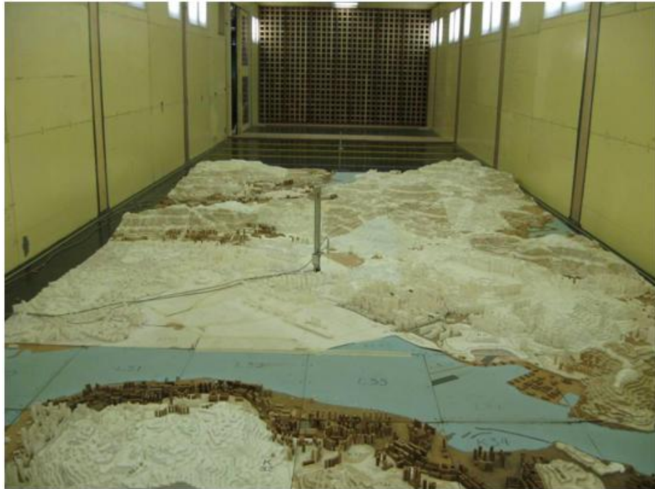
Figure 16 1:2000 scale topographical model in the low speed test section (Study Area A, north wind direction, 360°)
