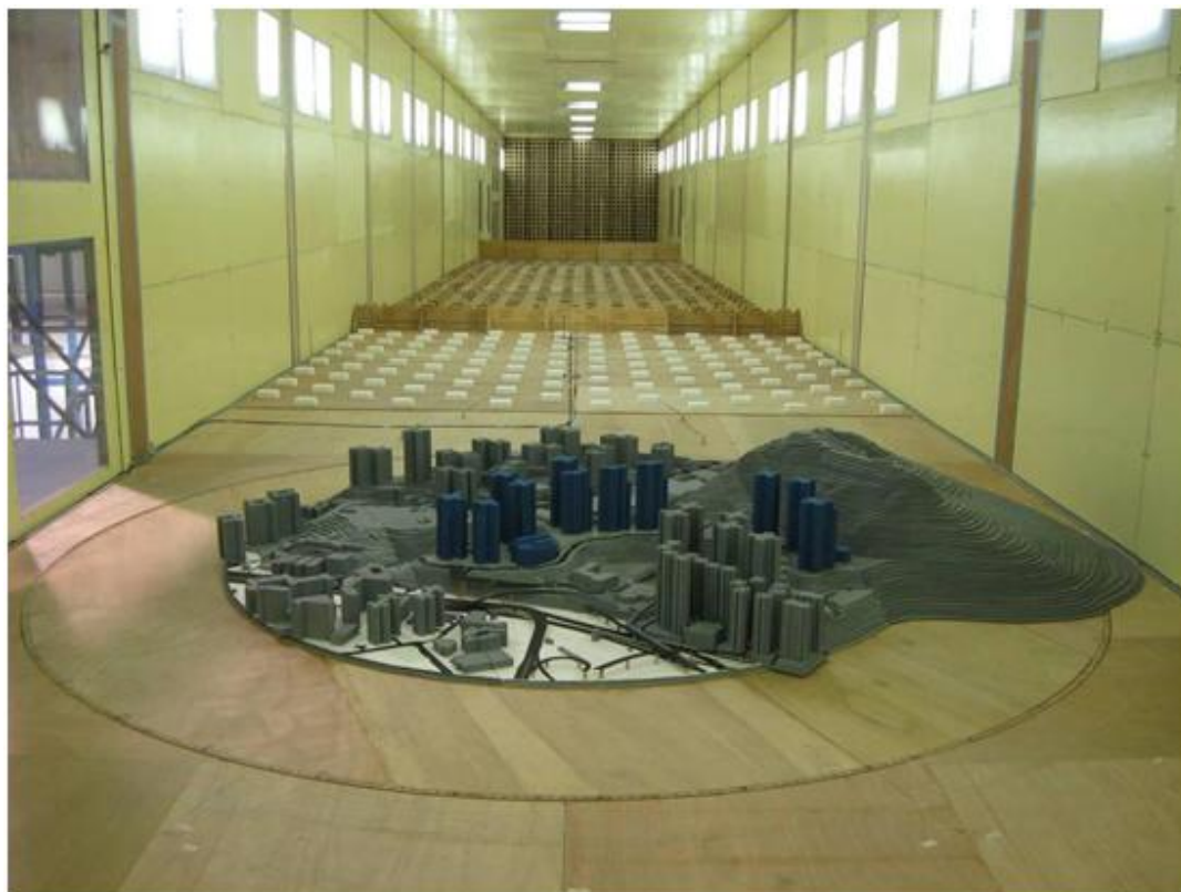
Figure 25 1:400 scale physical model of the Choi Wan Road Sites Study Area A and surrounds, Proposed Scheme, downstream view of north wind direction
