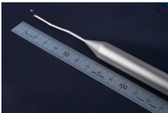
Figure 5 Hardware of the miniature dynamic pressure (Cobra) probe
