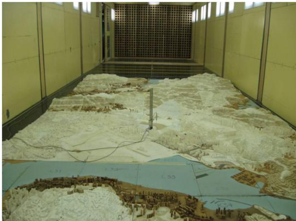
Figure 17 1:2000 scale topographical model in the low speed test section (Study Area B, north wind direction, 360°)
