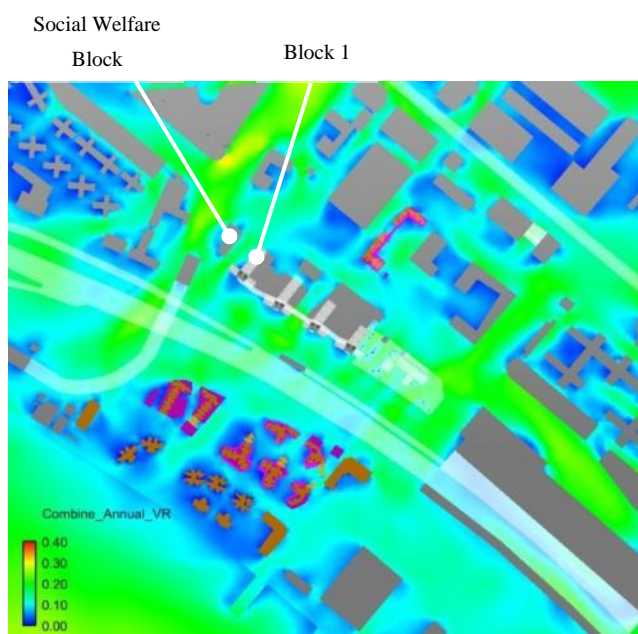
Figure A 1 Contour Plot of the average VR at 2m Pedestrian Level for Original Scheme and Further Enhanced Scheme – Annual Condition
