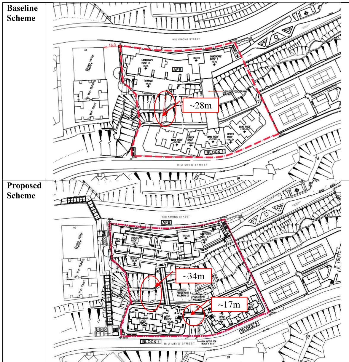
Figure 7 Building Separation (within Subject Site)
