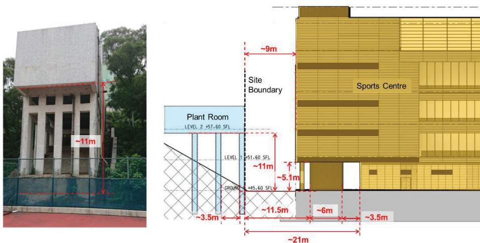
Figure 2.6 Schematic Section View of the Existing Plant Room and the Proposed Sports Centre under Proposed S16A Application Scheme
