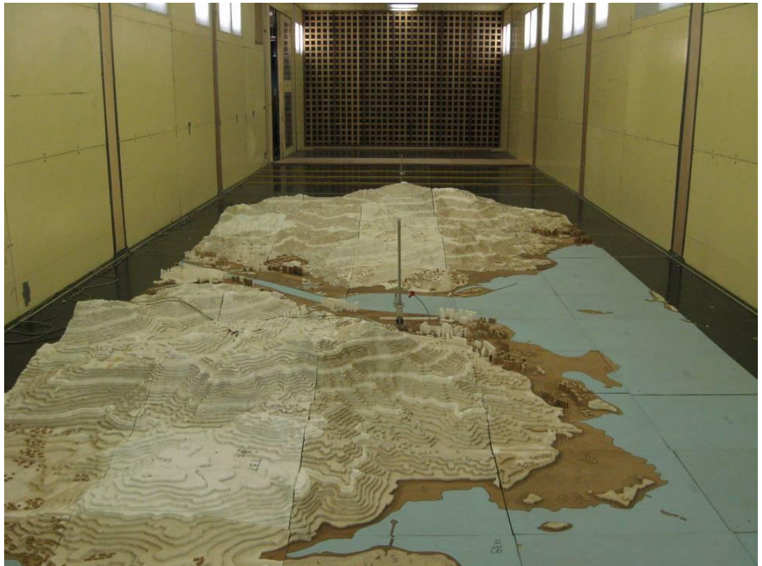
Figure 11 1:2000 scale topographical model in the low speed test section (west wind direction, 270°)
