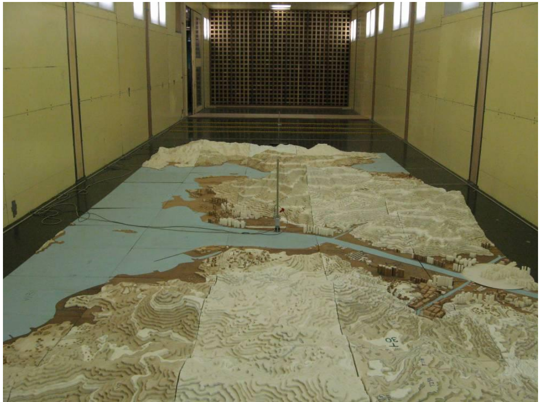
Figure 9 1:2000 scale topographical model in the low speed test section (east wind direction, 90°)
