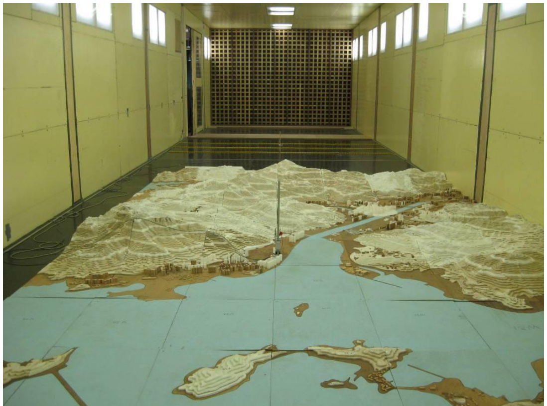
Figure 10 1:2000 scale topographical model in the low speed test section (south wind direction, 180°)
