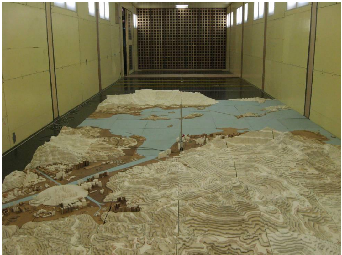
Figure 8 1:2000 scale topographical model in the low speed test section (north wind direction, 360°)
