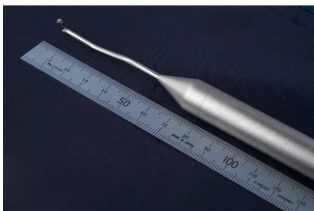
Figure 3 Hardware of the miniature dynamic pressure (Cobra) probe
