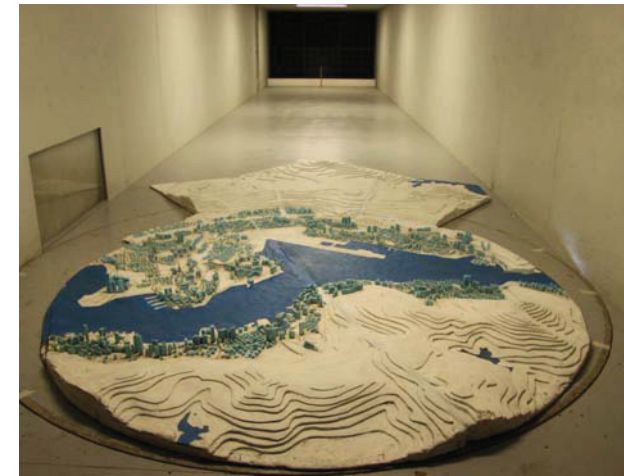
Figure 3a: Photograph of the topographic model in the wind tunnel (view from the north north east)
