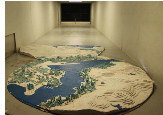
Figure 3b: Photograph of the topographic model in the wind tunnel (view from the east north east)
