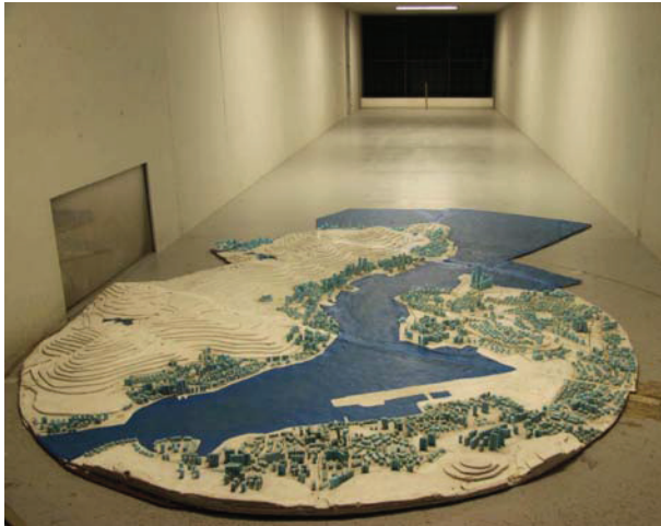
Figure 3c: Photograph of the topographic model in the wind tunnel (view from the west south west)
