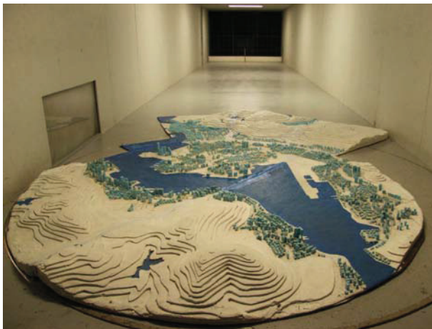
Figure 3d: Photograph of the topographic model in the wind tunnel (view from the north west)
