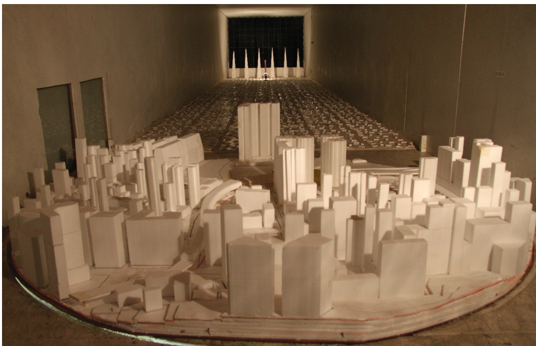
Figure 3h: Photograph of the Wind Tunnel Model – With Proposed Development (view from the east)
