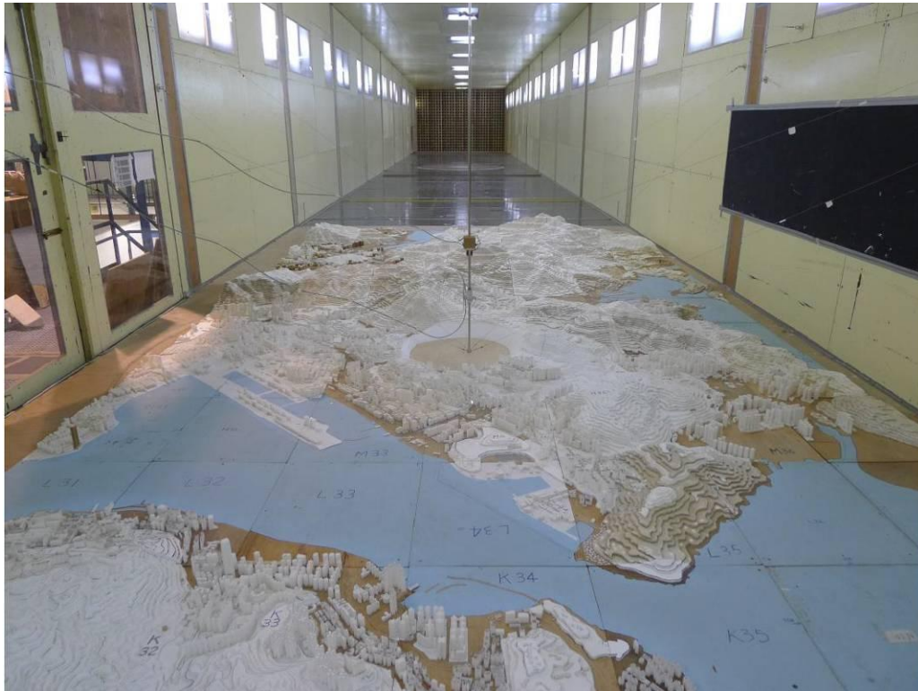
Figure 2.4 1:2000 scale topographical model of the Development at Anderson Road in the low speed test section (North wind direction, 360°)
