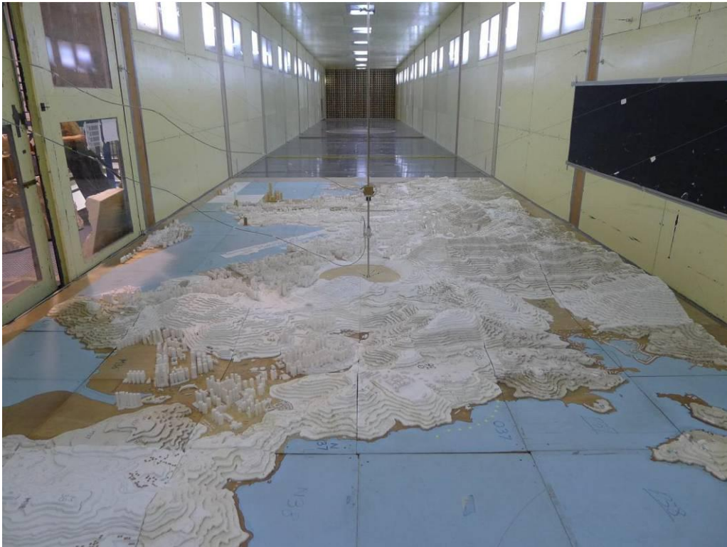
Figure 2.7 1:2000 scale topographical model of the Development at Anderson Road in the low speed test section (West wind direction, 270^{\circ} )
