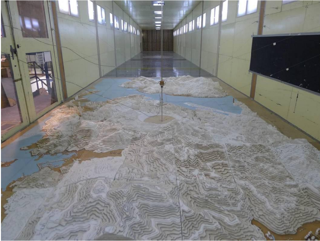
Figure 2.6 1:2000 scale topographical model of the Development at Anderson Road in the low speed test section (South wind direction, 180^{\circ} )
