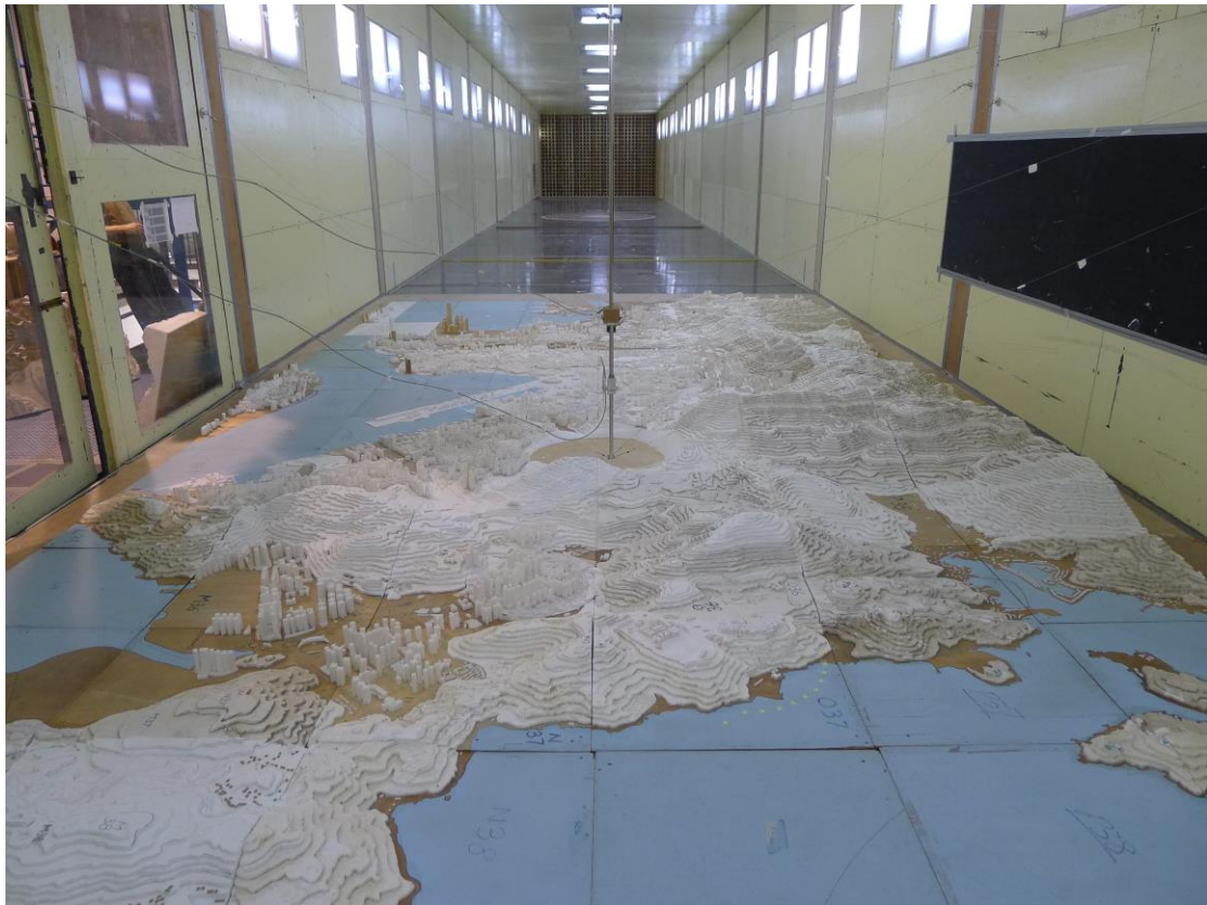
Figure 10: WWTF's 1:2000 topographical model of Hong Kong, 270° wind direction, downstream view.
