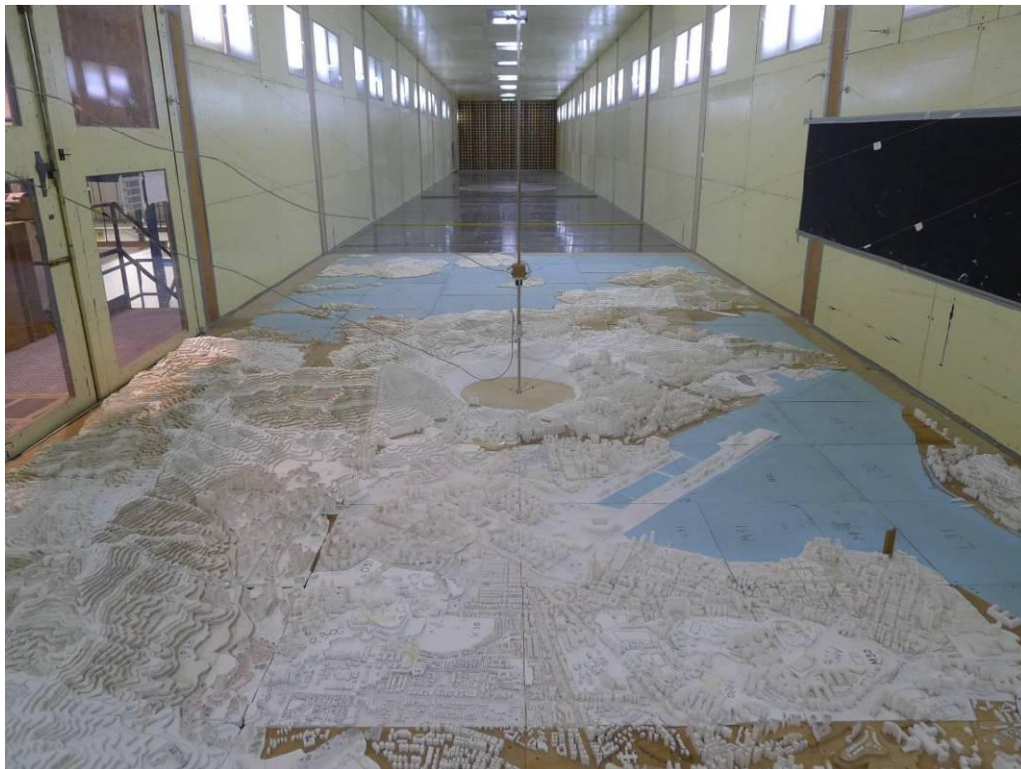
Figure 2.5 1:2000 scale topographical model of the Development at Anderson Road in the low speed test section (East wind direction, 90°)
