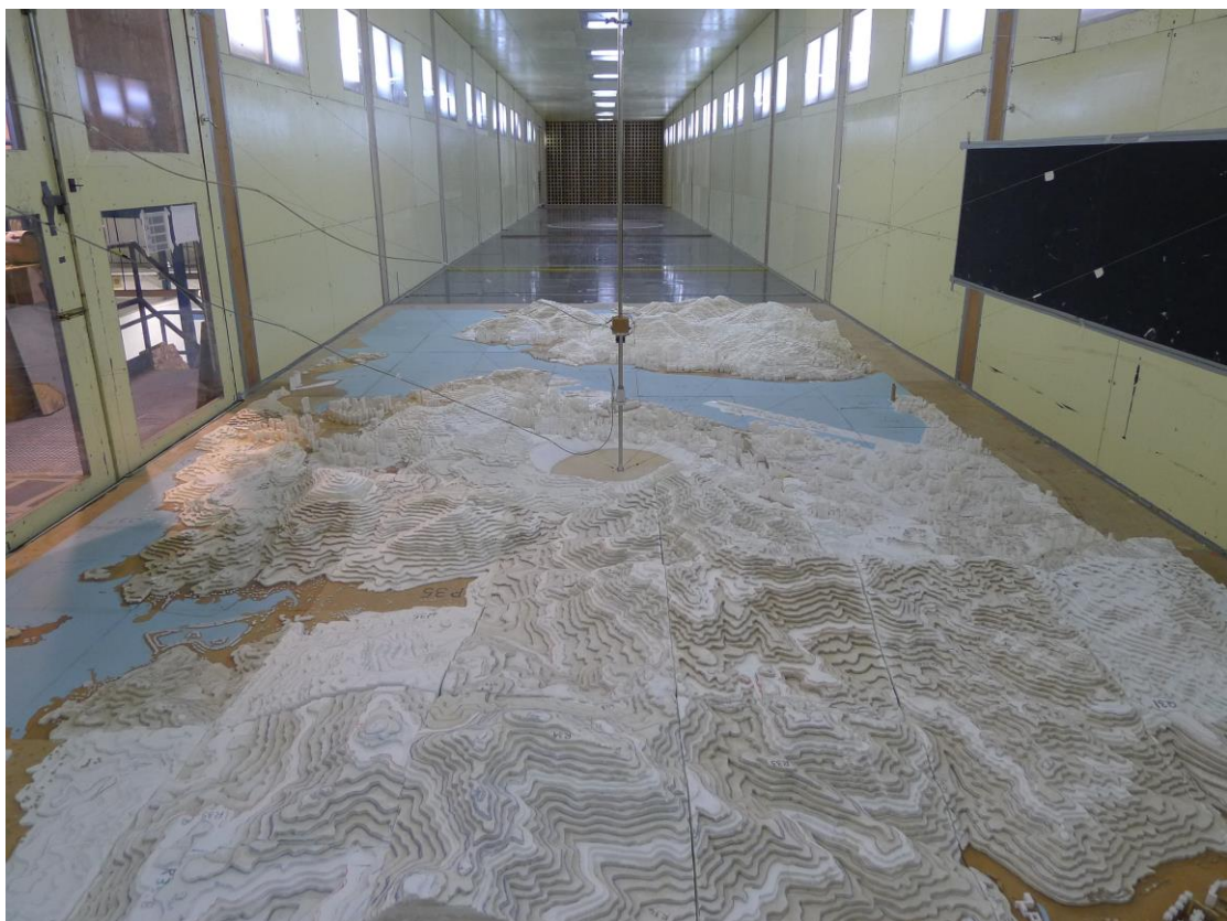
Figure 9: WWTF's 1:2000 topographical model of Hong Kong, 180° wind direction, downstream view.
