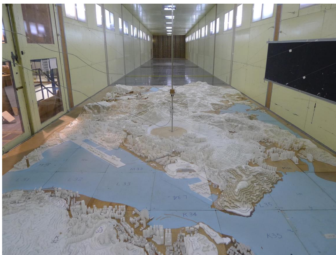
Figure 7: WWTF's 1:2000 topographical model of Hong Kong, 0° wind direction, downstream view.
