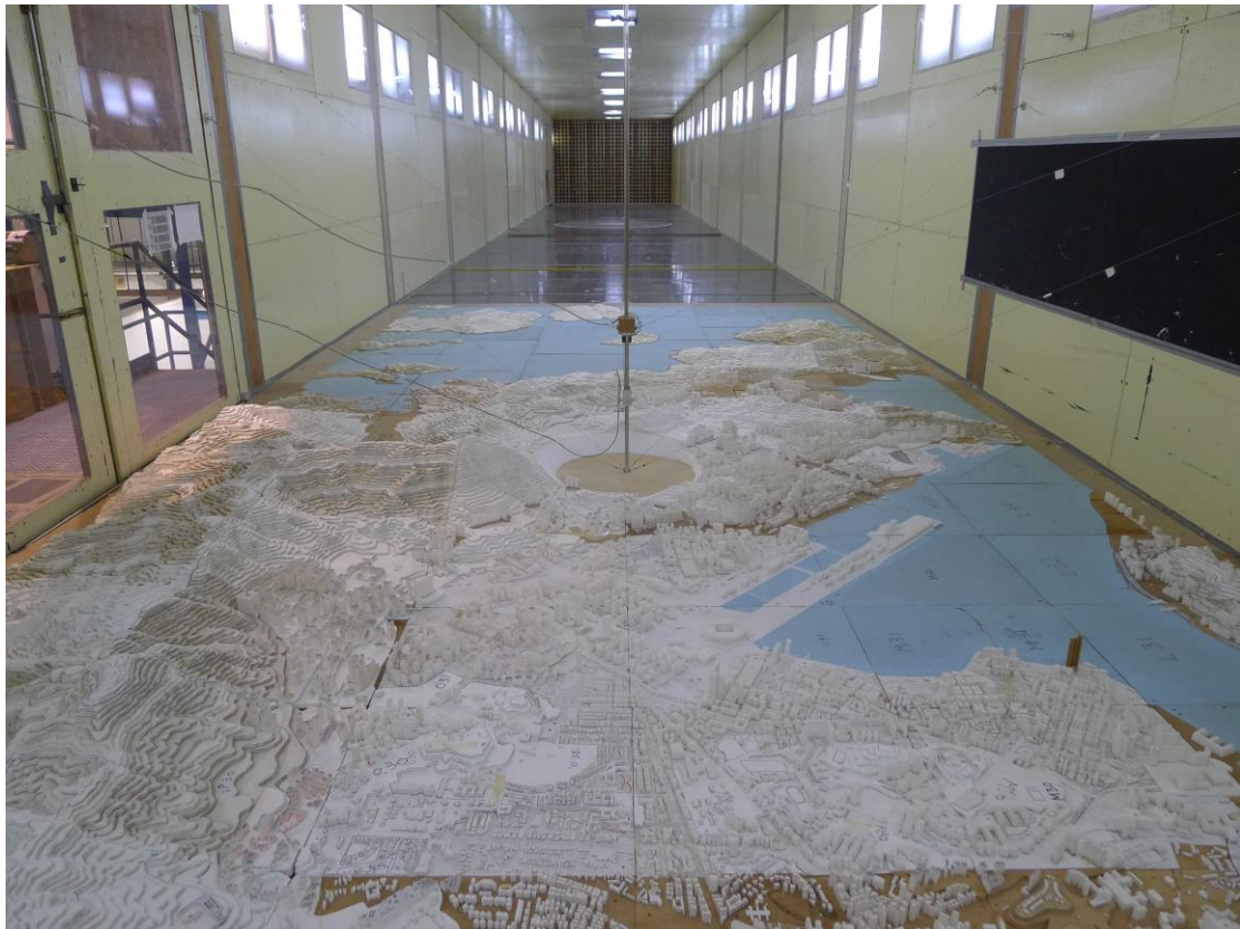
Figure 8: WWTF's 1:2000 topographical model of Hong Kong, 90° wind direction, downstream view.
