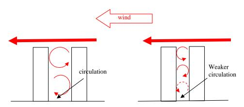
Figure 7.2 Circulation between buildings for wider & narrower gaps
