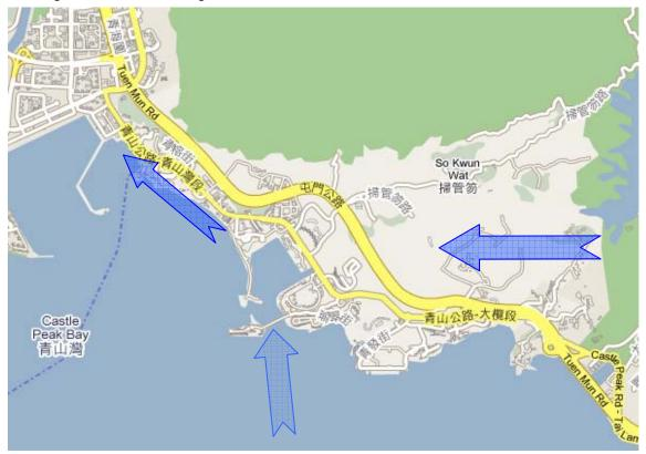
Figure 6.10b Prevailing flow directions in Tuen Mun East Area summer condition
