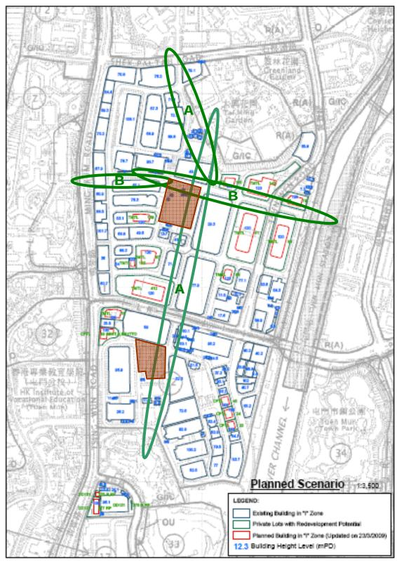
(Building layouts for redevelopment sites are indicative only and are prepared for AVA EE Assessment purpose) Figure 7.1 Flow paths and locations for set-backs & building gaps for Industrial area
