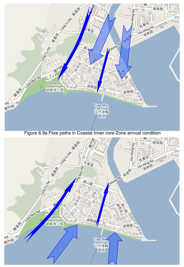
Figure 6.9b Flow paths in Coastal Inner core Zone summer condition
