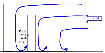
Figure 6.2b Downwash wind for buildings with progressively increasing heights
