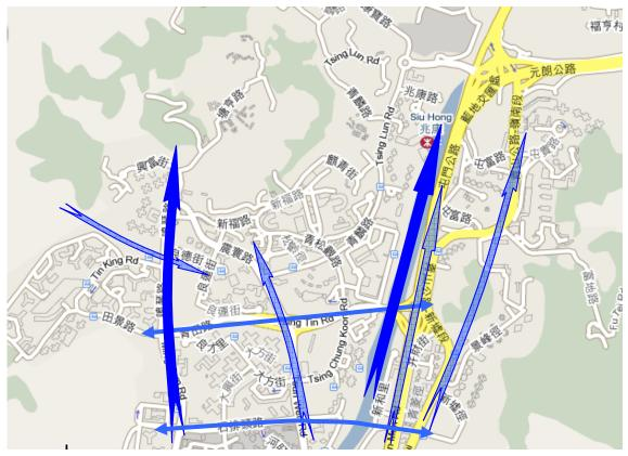
Figure 6.6b Flow paths in Northern Inner core Zone summer condition
