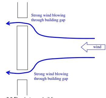
Figure 6.3 Flow between building gaps
