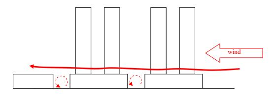
Figure 7.3 Wind forced to blow over podiums
