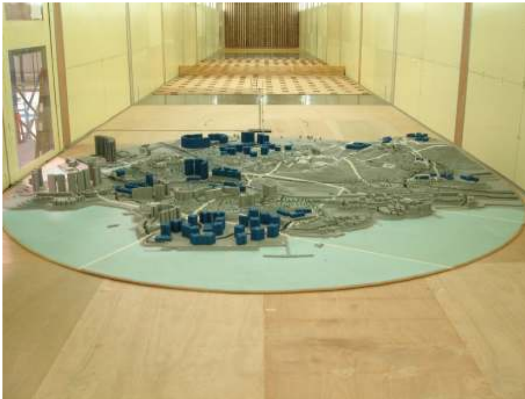
Figure 19: 1:400 scale East Model of the Tuen Mun East Study Area, wind direction = 0°
