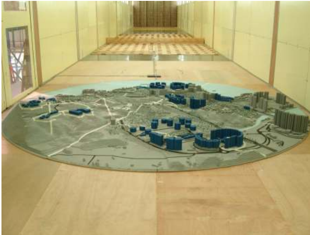
Figure 21: 1:400 scale East Model of the Tuen Mun East Study Area, wind direction = 180°
