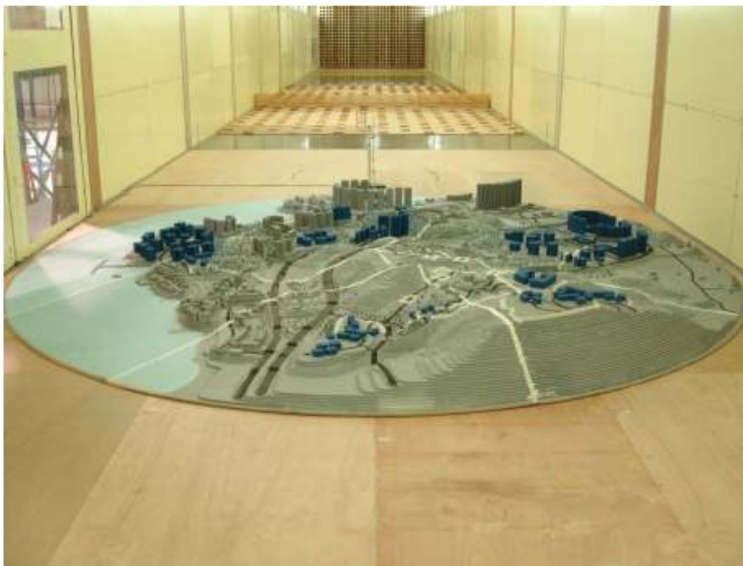
Figure 22: 1:400 scale East Model of the Tuen Mun East Study Area, wind direction = 270°
