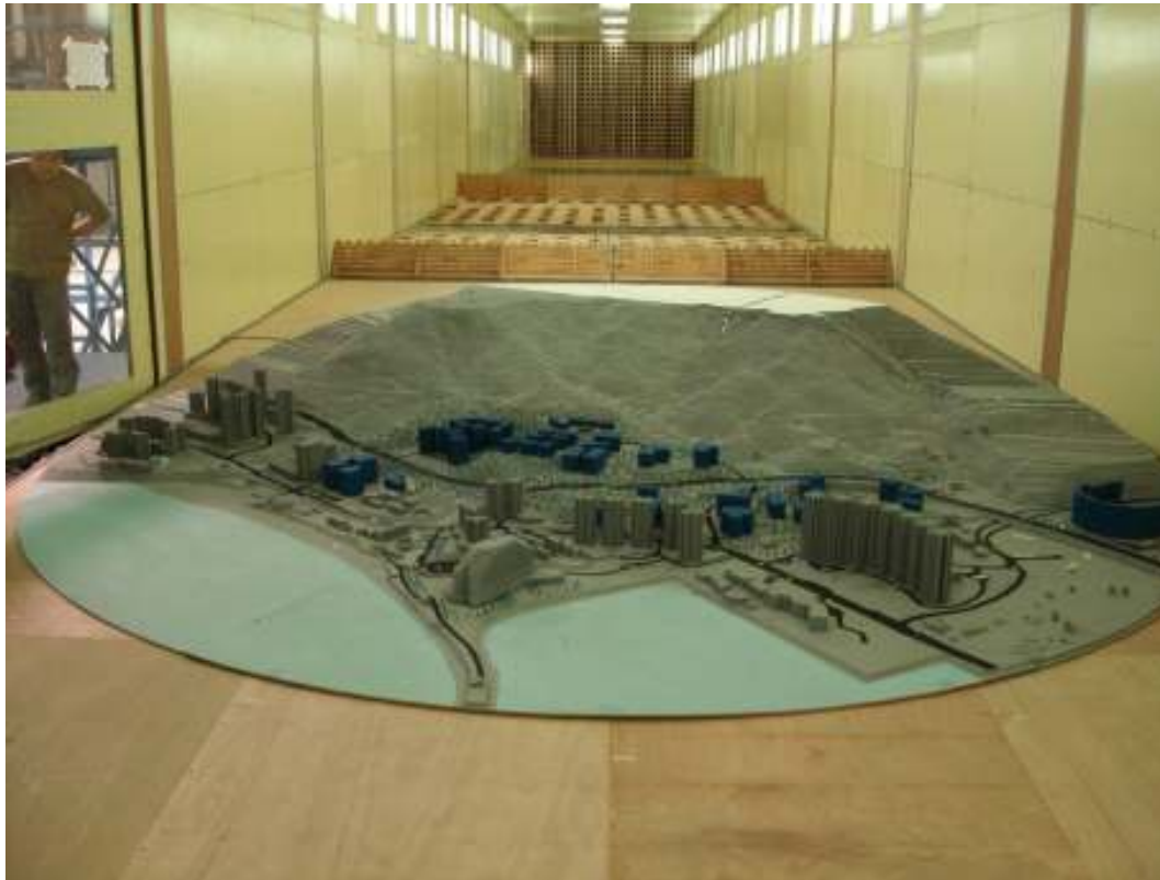
Figure 23: 1:400 scale West Model of the Tuen Mun East Study Area, wind direction = 0°
