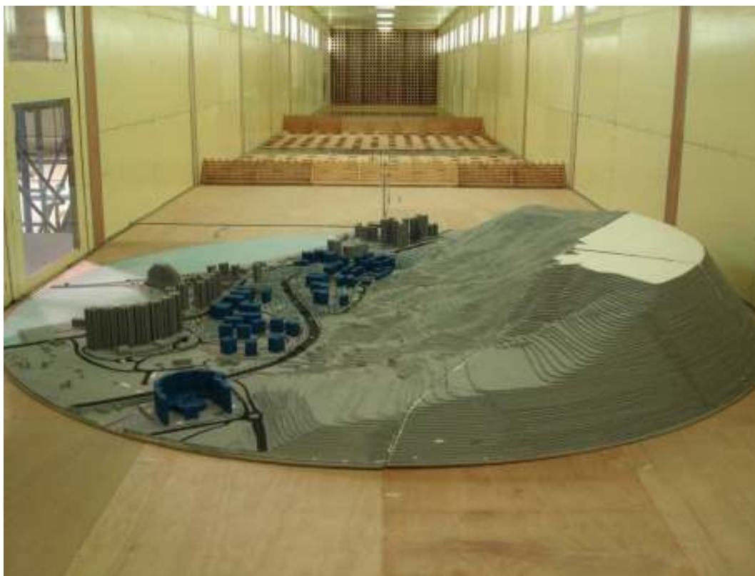
Figure 26: 1:400 scale West Model of the Tuen Mun East Study Area, wind direction = 270°
