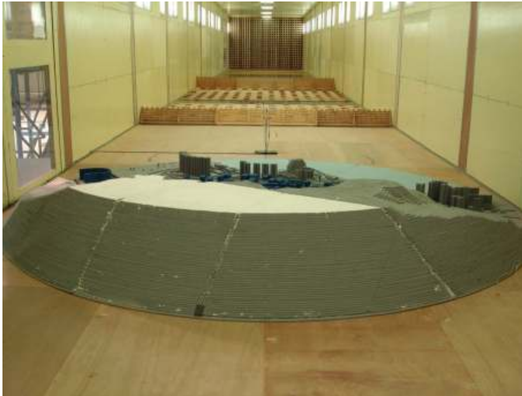
Figure 25: 1:400 scale West Model of the Tuen Mun East Study Area, wind direction = 180°
