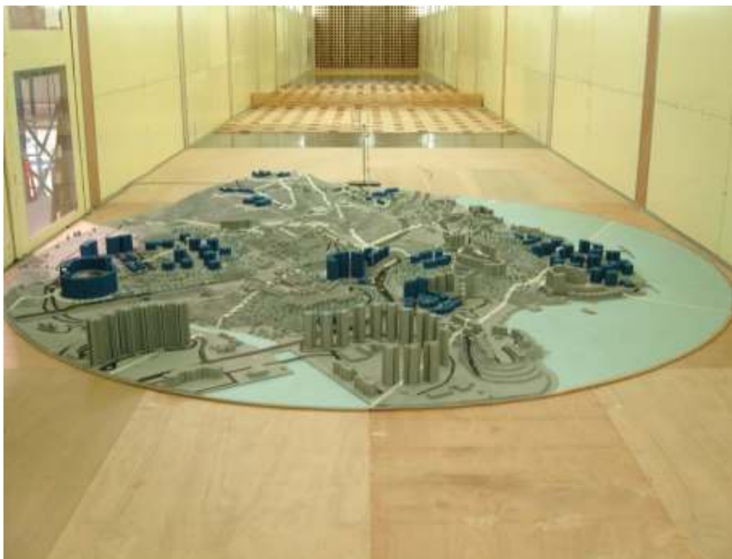
Figure 20: 1:400 scale East Model of the Tuen Mun East Study Area, wind direction = 90°
