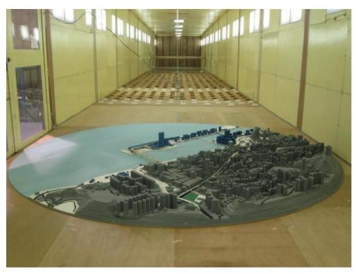
Figure 16: A 1:800 scale model of the proposed Kai Tak Development in the low speed test section, Study Area A, (west wind direction, 270°)
