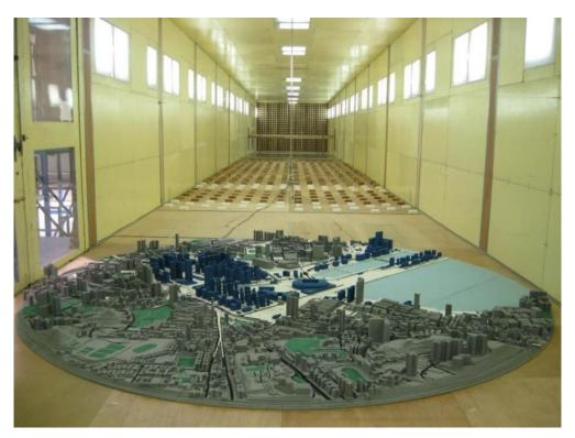
Figure 18: A 1:800 scale model of the proposed Kai Tak Development in the low speed test section, Study Area B, (east wind direction, 90°)
