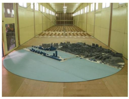
Figure 13: A 1:800 scale model of the proposed Kai Tak Development in the low speed test section, Study Area A, (north wind direction, 0°)
