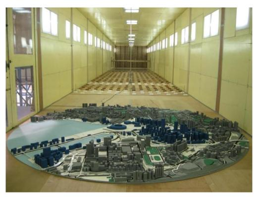
Figure 20: A 1:800 scale model of the proposed Kai Tak Development in the low speed test section, Study Area B, (west wind direction, 270°)
