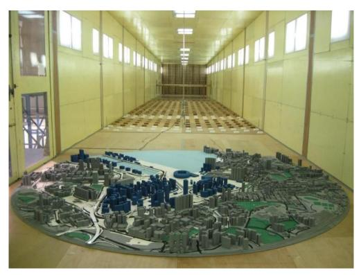
Figure 19: A 1:800 scale model of the proposed Kai Tak Development in the low speed test section, Study Area B, (south wind direction, 180°)
