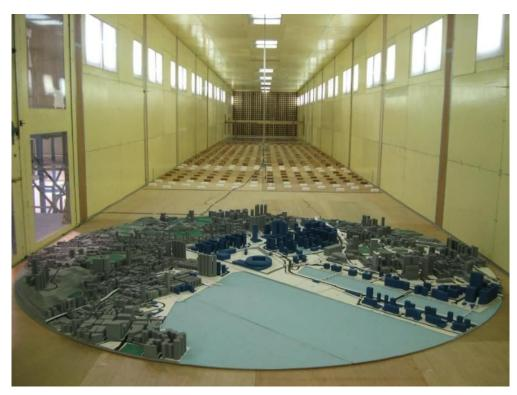
Figure 17: A 1:800 scale model of the proposed Kai Tak Development in the low speed test section, Study Area B, (north wind direction, 0°)
