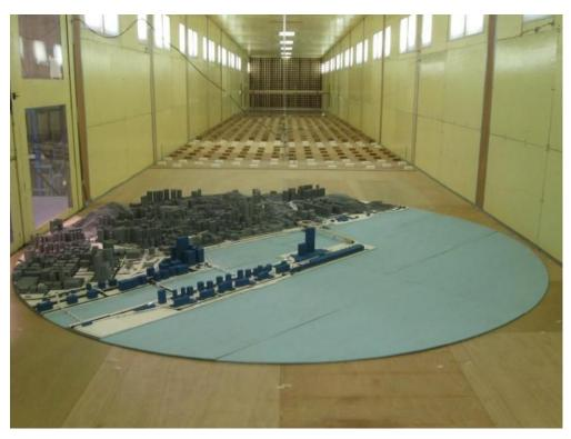
Figure 14: A 1:800 scale model of the proposed Kai Tak Development in the low speed test section, Study Area A, (east wind direction, 90°)
