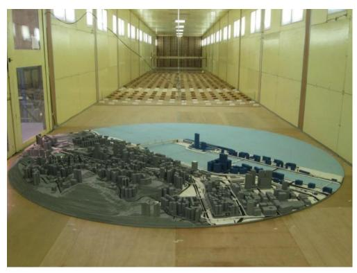
Figure 15: A 1:800 scale model of the proposed Kai Tak Development in the low speed test section, Study Area A, (south wind direction, 180°)
