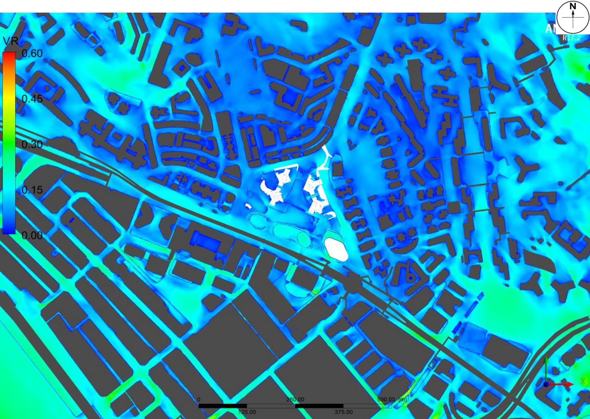
Baseline Scheme - Summer weighted wind speed colour at pedestrian level
