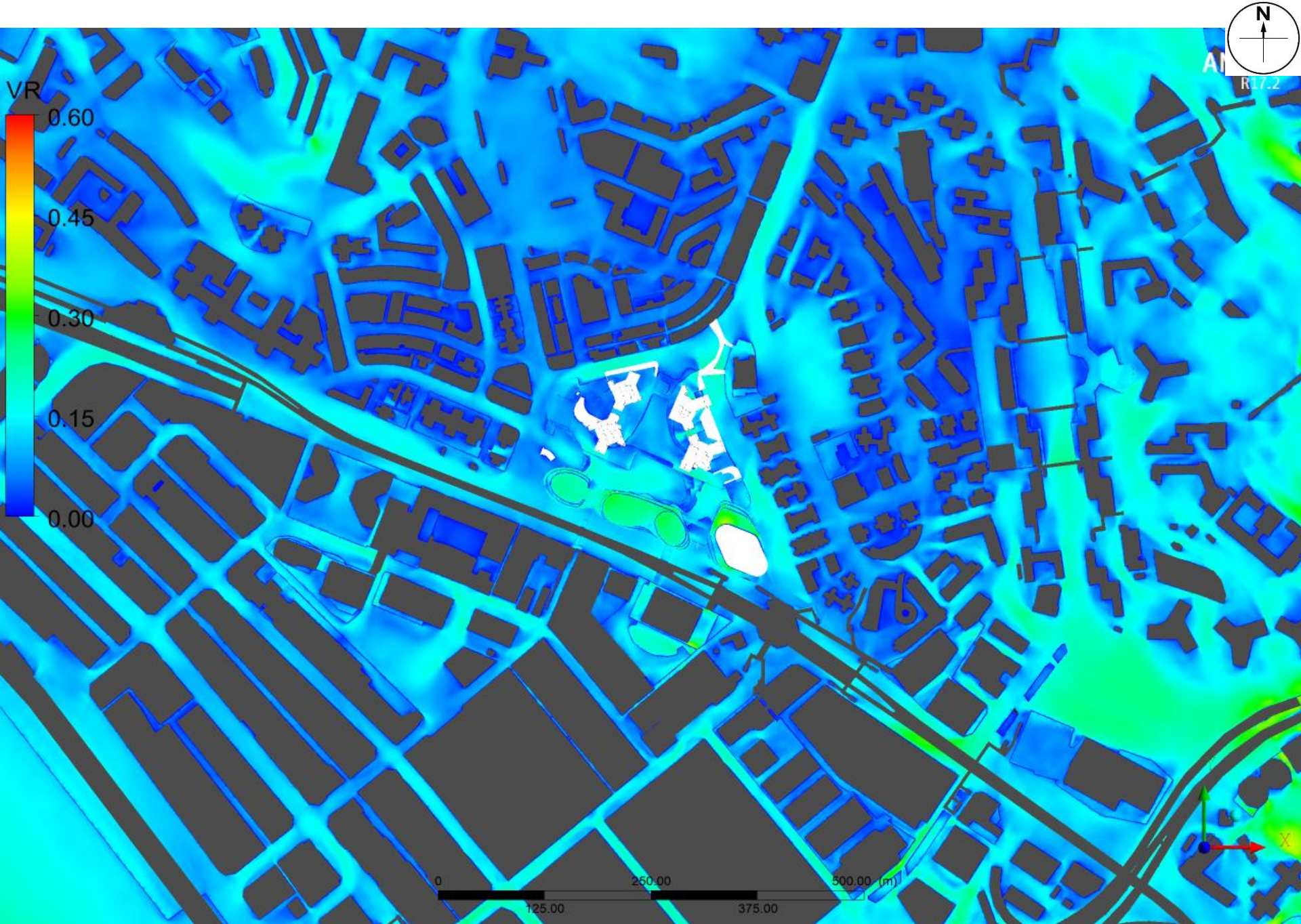
Baseline Scheme - Annual weighted wind speed colour at pedestrian level
