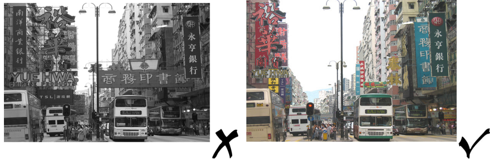
Figure 54 Projecting Signboards should be Vertical Type instead of Horizontal Type
