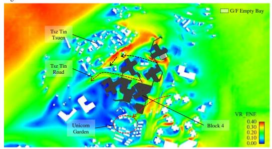
Figure 28 VR Contour Plot for Proposed Scheme under ENE Wind
