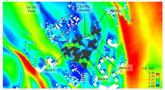
Figure 34 VR Contour Plot for Proposed Scheme under SSE Wind
