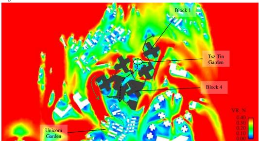
Figure 22 VR Contour Plot for Proposed Scheme under N Wind
