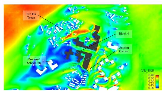
Figure 27 VR Contour Plot for Baseline Scheme under ENE Wind
