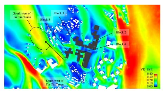
Figure 33 VR Contour Plot for Baseline Scheme under SSE Wind
