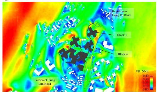
Figure 24 VR Contour Plot for Proposed Scheme under NNE Wind
