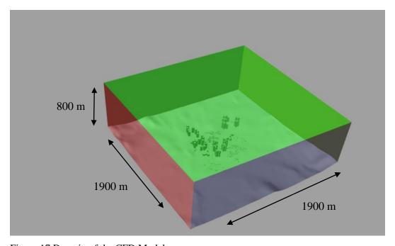
Figure 17 Domain of the CFD Model
