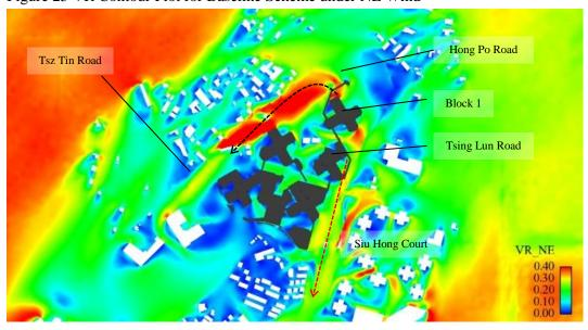
Figure 26 VR Contour Plot for Proposed Scheme under NE Wind
