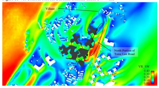
Figure 36 VR Contour Plot for Proposed Scheme under SW Wind
