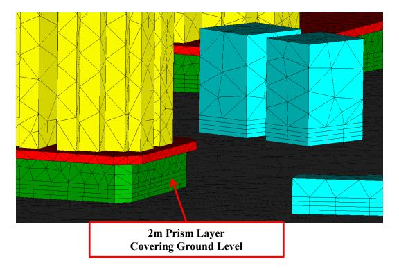
Figure 18 Prism Layer of the CFD Model
