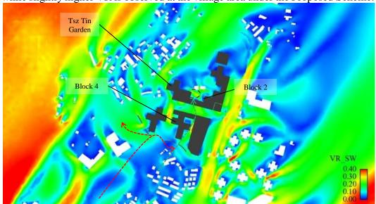
Figure 35 VR Contour Plot for Baseline Scheme under SW Wind
