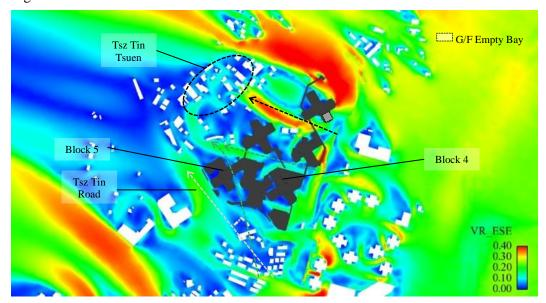
Figure 32 VR Contour Plot for Proposed Scheme under ESE Wind
