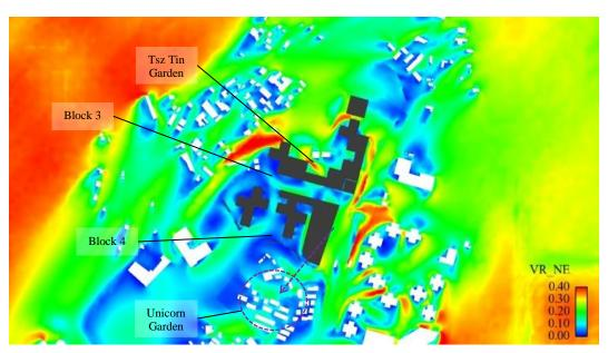
Figure 25 VR Contour Plot for Baseline Scheme under NE Wind
