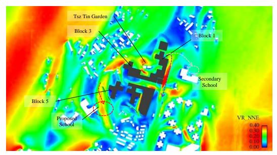
Figure 23 VR Contour Plot for Baseline Scheme under NNE Wind
