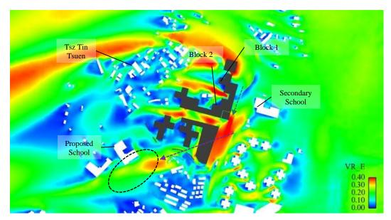
Figure 29 VR Contour Plot for Baseline Scheme under E Wind
