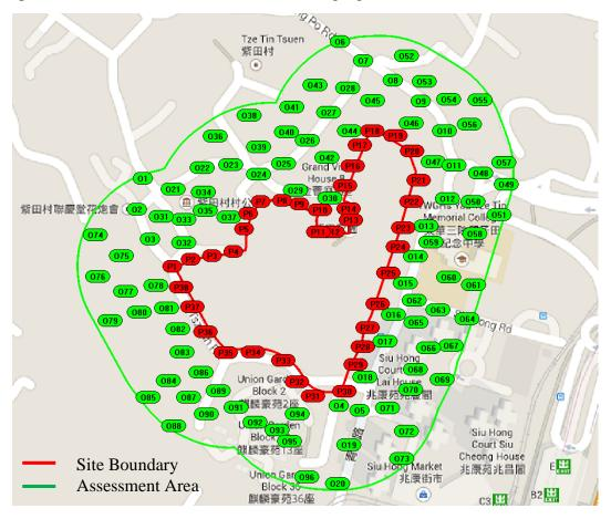
Figure 16 Demarcation of Test Points for Site Air Ventilation Assessment
