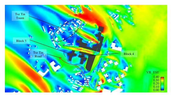
Figure 31 VR Contour Plot for Baseline Scheme under ESE Wind
