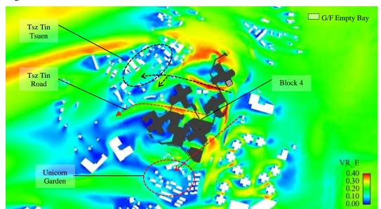
Figure 30 VR Contour Plot for Proposed Scheme under E Wind
