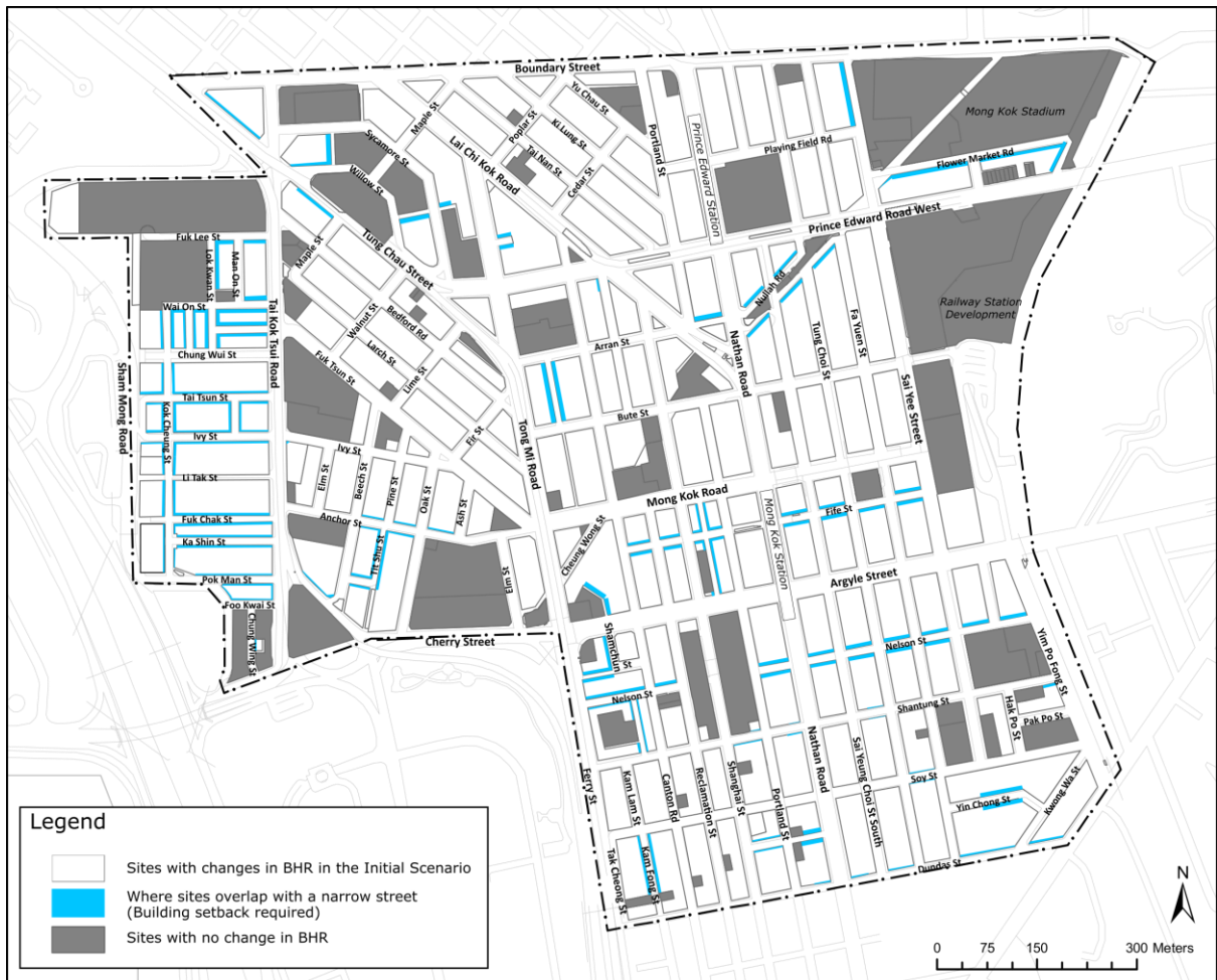
Figure 6.6 Building sites fronting narrow streets < 15m wide which should adopt SB as required by the SBDG in MK Area.
