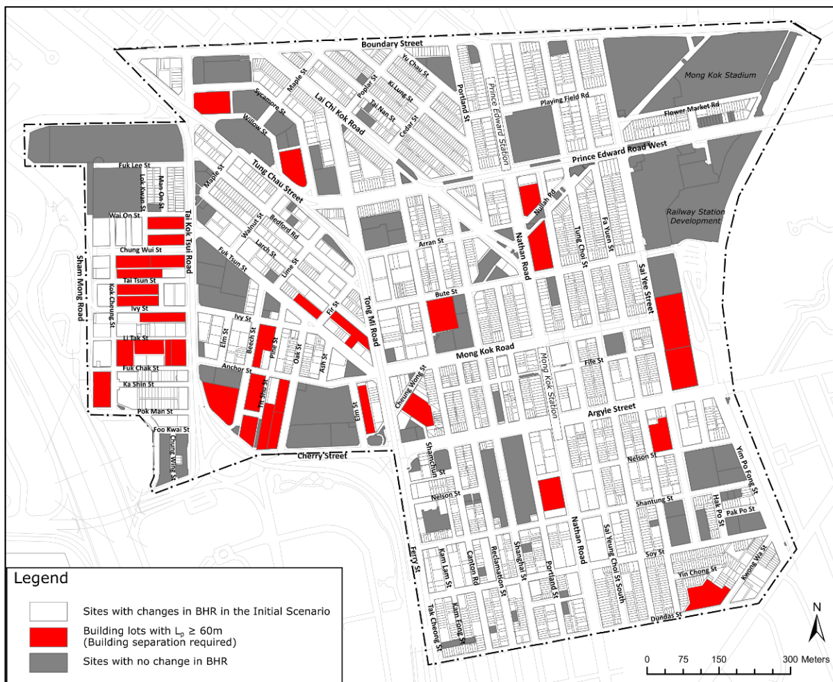
Figure 6.7 Existing building lots with \geq 60m which should adopt building separation as required by the SBDG in MK Area.
