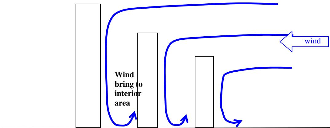
Figure 6.2b Downwash wind for buildings with progressively increasing heights
