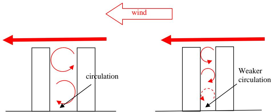
Figure 7.2 Circulation between buildings for wider & narrower gaps
