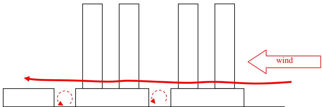
Figure 7.3 Wind forced to blow over podiums
