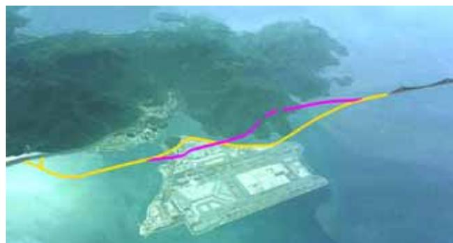
*Different possible alignments for the proposed HZMB and North Lantau Highway Connection*
