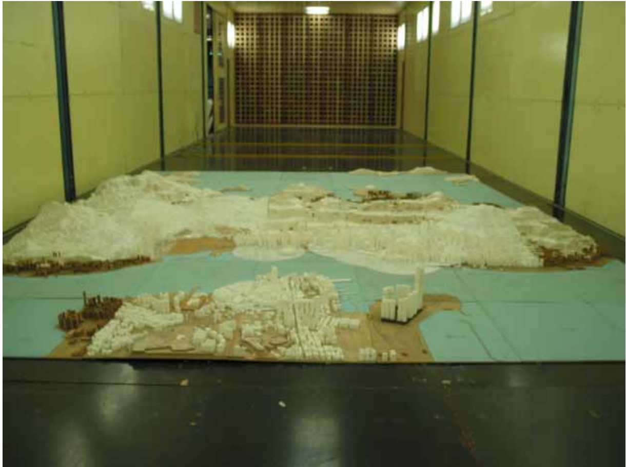
Figure 7: A 1:2000 scale topographical model of Causeway Bay, Hong Kong in the low speed test section of the CLP Power Wind/Wave Tunnel Facility (south wind direction, 180°)
