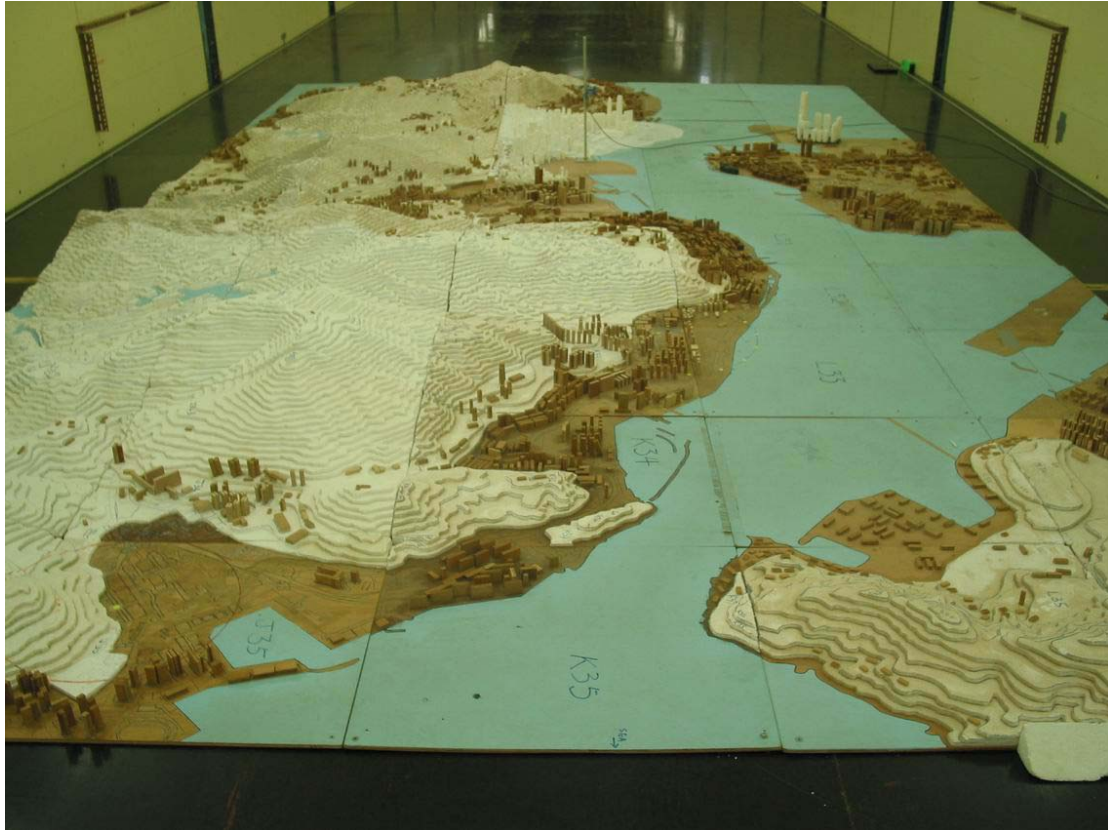
Figure 6: A 1:2000 scale topographical model of the Central Waterfront, Hong Kong in the low-speed test section of the CLP Power Wind/Wave Tunnel Facility (East wind direction, 90°)
