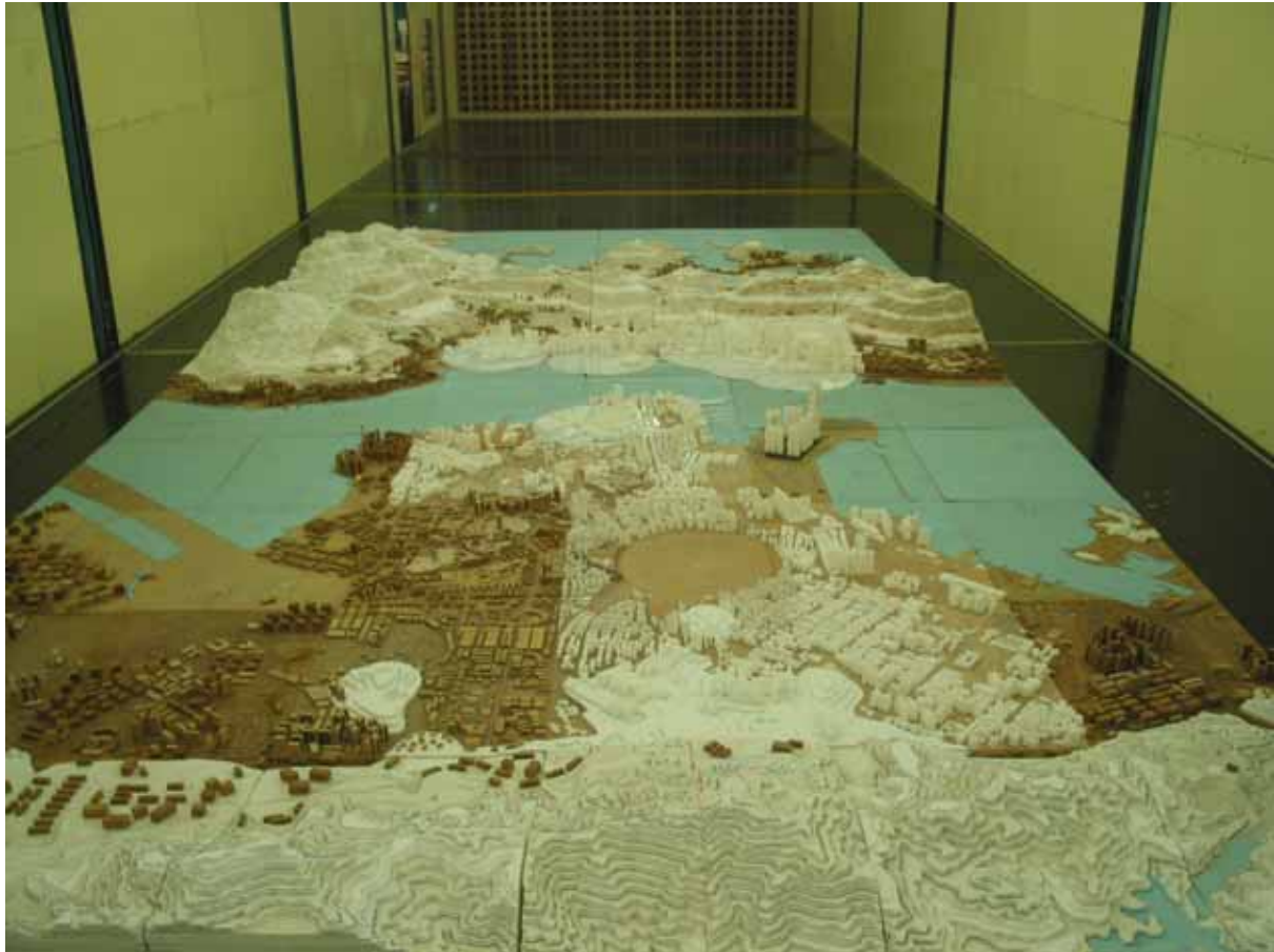
Figure 7: A 1:2000 scale topographical model of Mong Kok, Hong Kong in the low speed test section of the CLP Power Wind/Wave Tunnel Facility (south wind direction, 180°)
