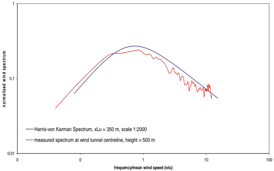
Figure 6: Longitudinal turbulence spectrum – approach wind
