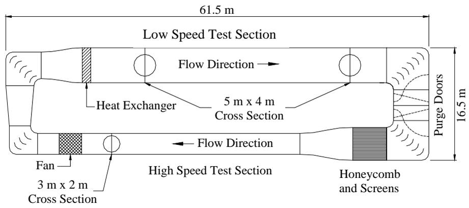
Figure 4: Test sections at the CLP Power Wind/Wave Tunnel Facility
