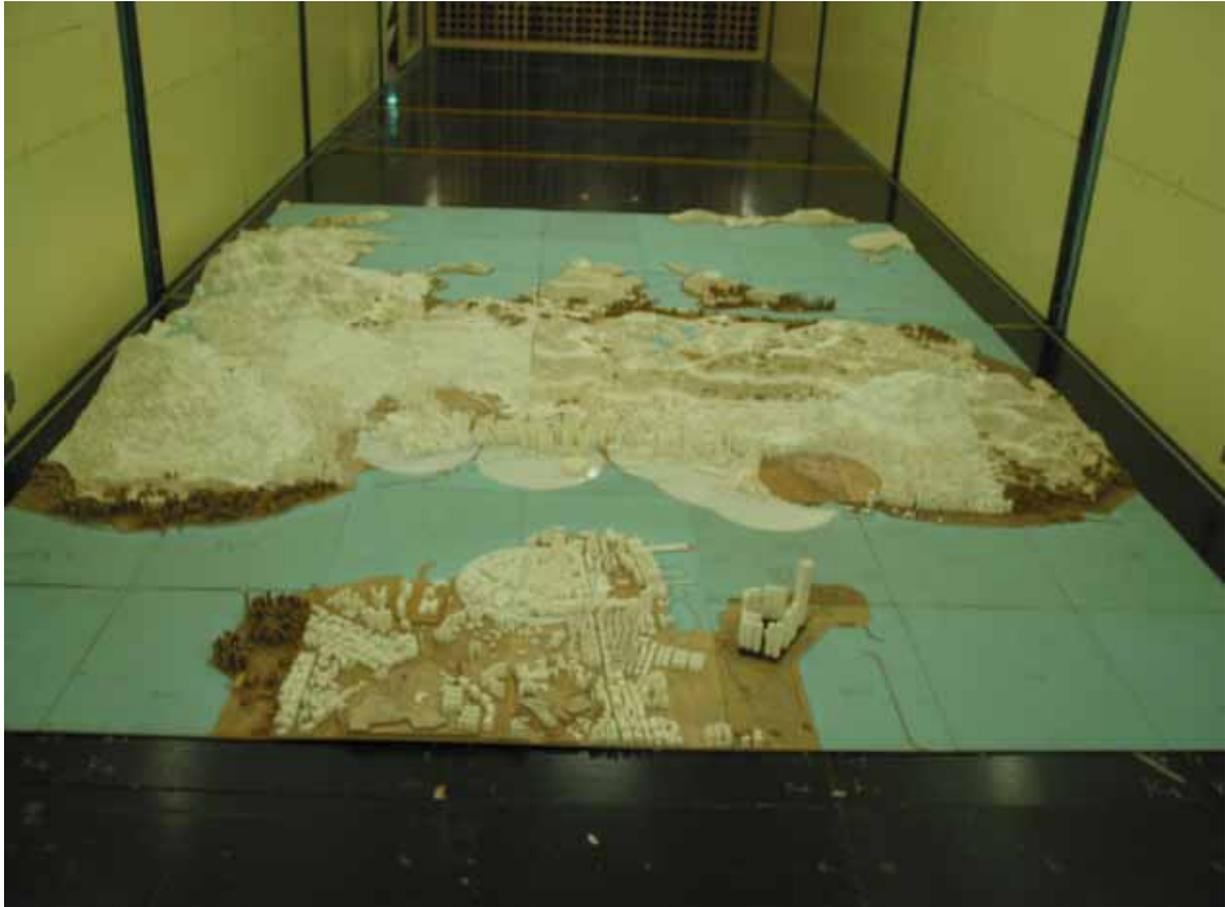
Figure 7: A 1:2000 scale topographical model of Sheung Wan, Hong Kong in the low speed test section of the CLP Power Wind/Wave Tunnel Facility (south wind direction, 180°)
