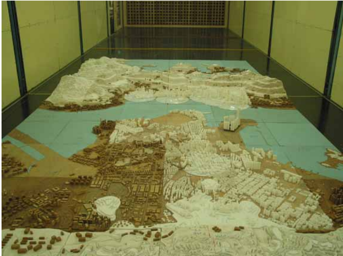
Figure 7: A 1:2000 scale topographical model of Tsim Sha Tsui, Hong Kong in the low speed test section of the CLP Power Wind/Wave Tunnel Facility (south wind direction, 180°)
