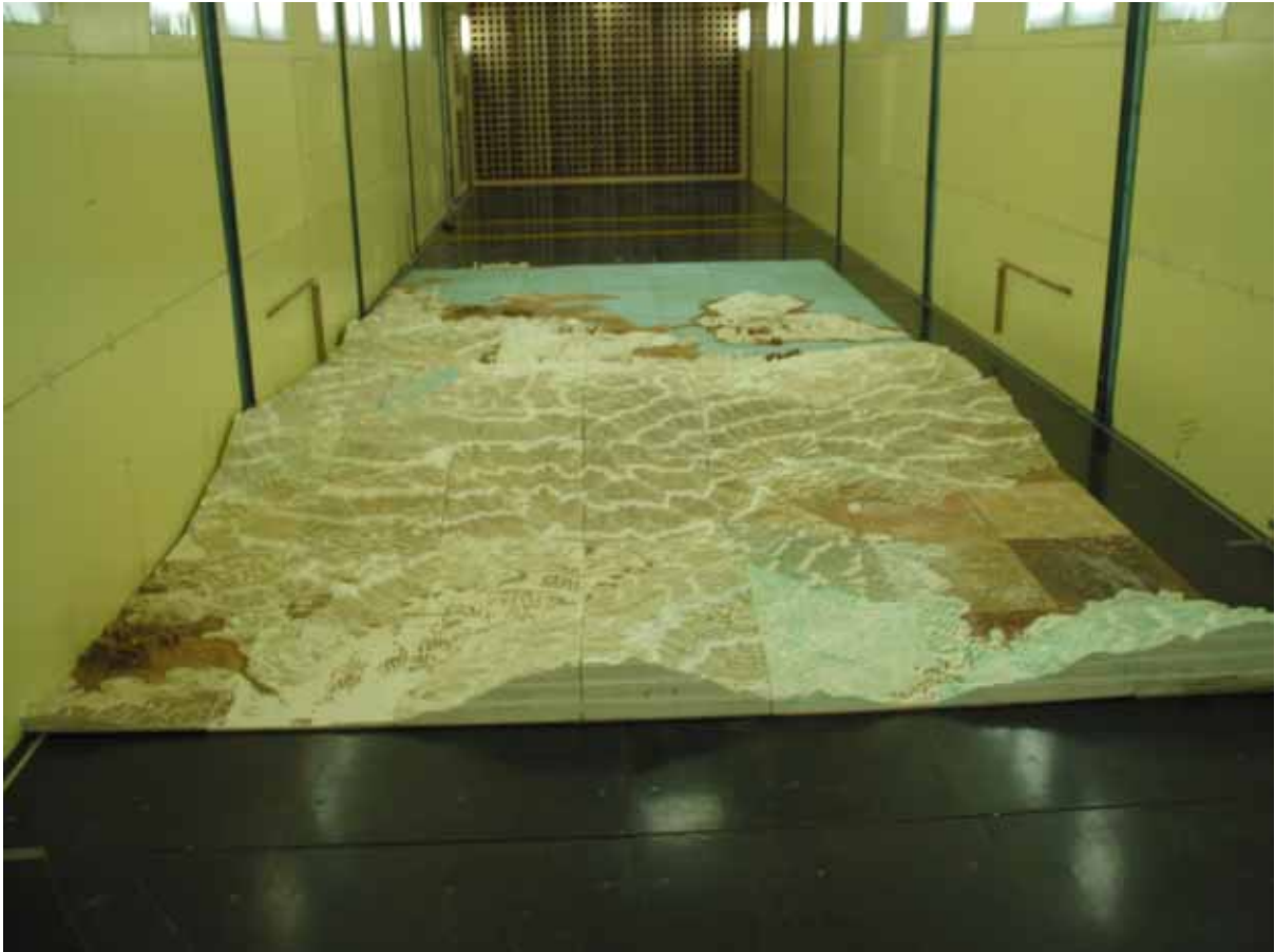
Figure 7: A 1:2000 scale topographical model of Tsuen Wan, Hong Kong in the low speed test section of the CLP Power Wind/Wave Tunnel Facility (south wind direction, 180°)
