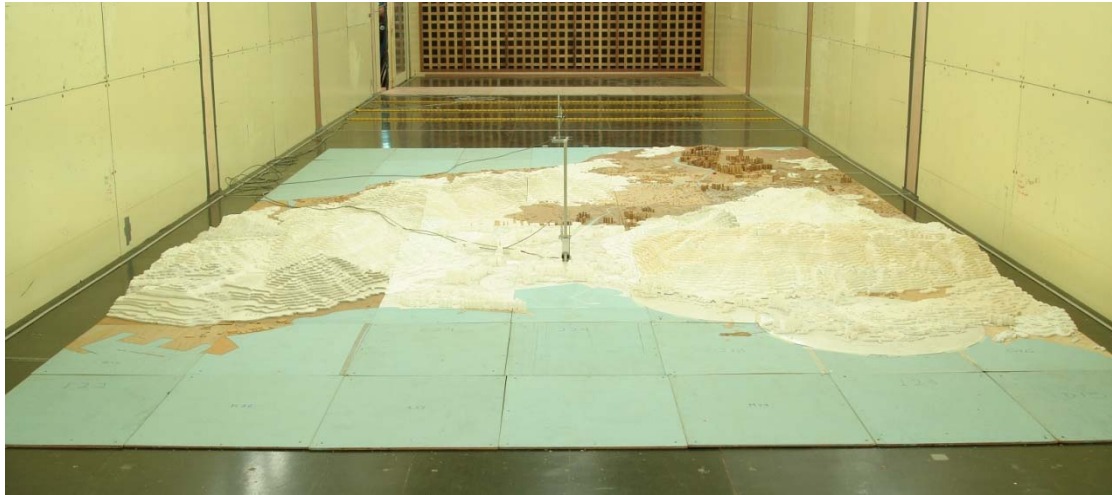
Figure 8: 1:2000 scale topographical model of Tuen Mun in the low speed test section of the CLP Power Wind/Wave Tunnel Facility (north wind direction, 360^\circ )
