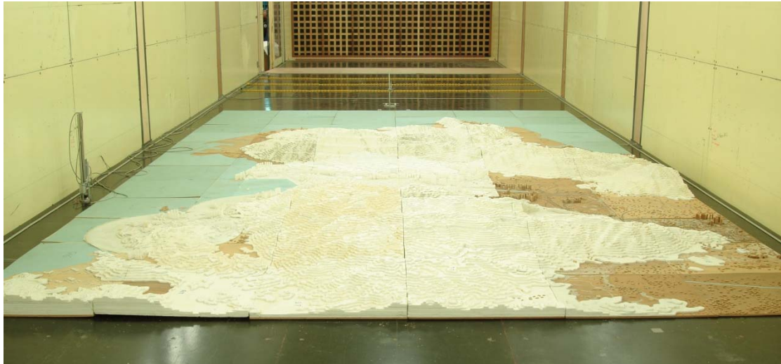
Figure 11: scale topographical model of Tuen Mun in the low speed test section of the CLP Power Wind/Wave Tunnel Facility (west wind direction, 270°)
