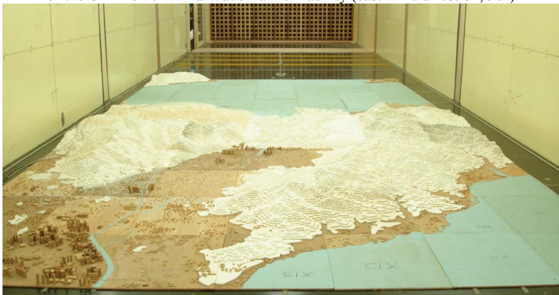
Figure 10: 1:2000 scale topographical model of Tuen Mun in the low speed test section of the CLP Power Wind/Wave Tunnel Facility (south wind direction, 180^\circ )
