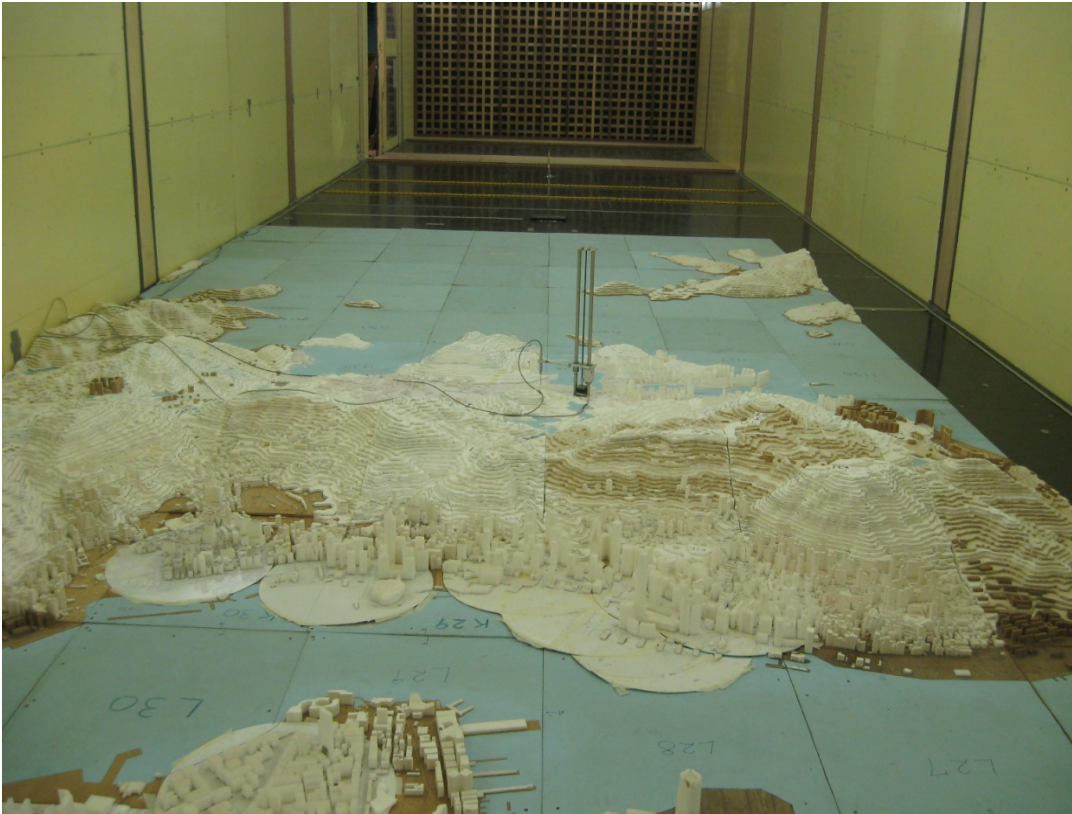
Figure 10: 1:2000 scale topographical model of Wong Chuk Hang in the low speed test section of the CLP Power Wind/Wave Tunnel Facility (south wind direction, 180°)
