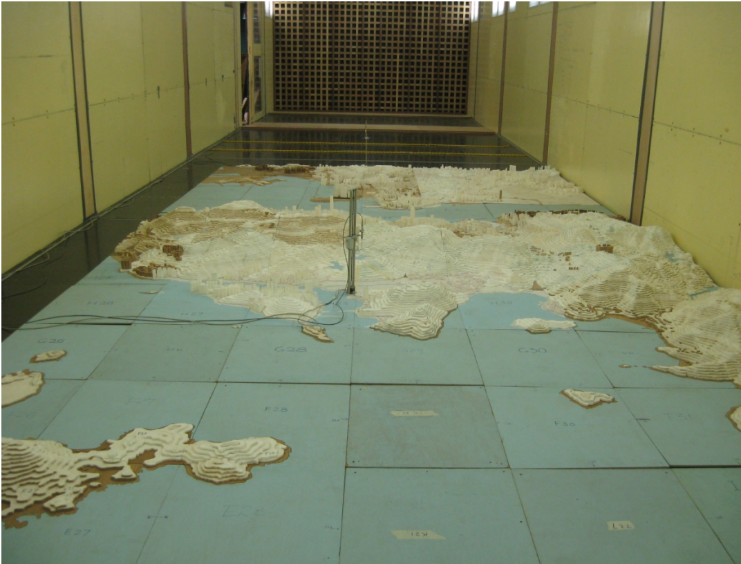
Figure 8: 1:2000 scale topographical model of Wong Chuk Hang in the low speed test section of the CLP Power Wind/Wave Tunnel Facility (north wind direction, 360°)
