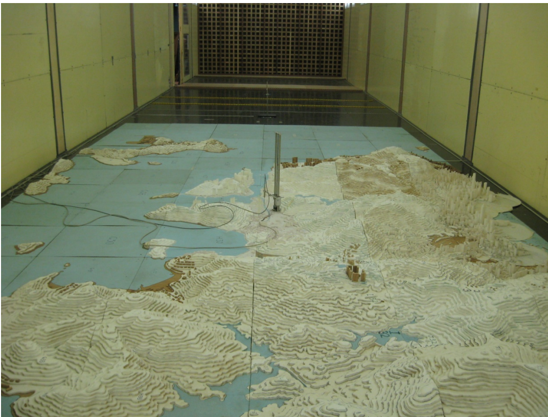
Figure 11: scale topographical model of Wong Chuk Hang in the low speed test section of the CLP Power Wind/Wave Tunnel Facility (west wind direction, 270°)
