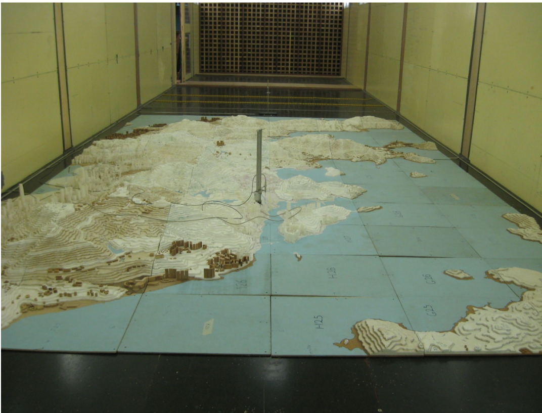
Figure 9: 1:2000 scale topographical model of Wong Chuk Hang in the low speed test section of the CLP Power Wind/Wave Tunnel Facility (east wind direction, 90°)
